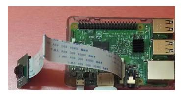
The Camera Module is a great accessory for the Raspberry Pi, allowing users to take still pictures and record video in full HD. Connect the **Camera Module** to the Raspberry Pi's camera port (Blue side of cable to face Ethernet connection).
