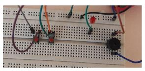
**The buzzer** is used to generate sound when button pressed.
